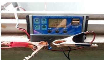
Gambar 10. Solarcharge controler
